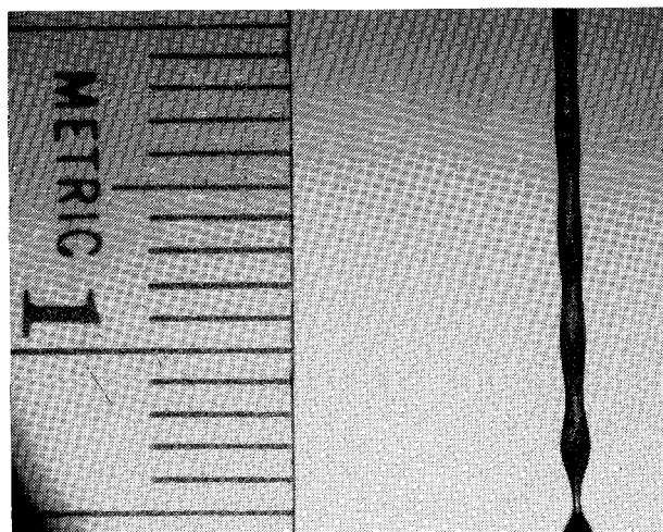
Fig. 9 Slurry jet. V_0 = 142 cm/s, \ell = 1.10 g/cm 3 , We = 16 , f = 431 Hz, \lambda/D_0 = 4.5 .
